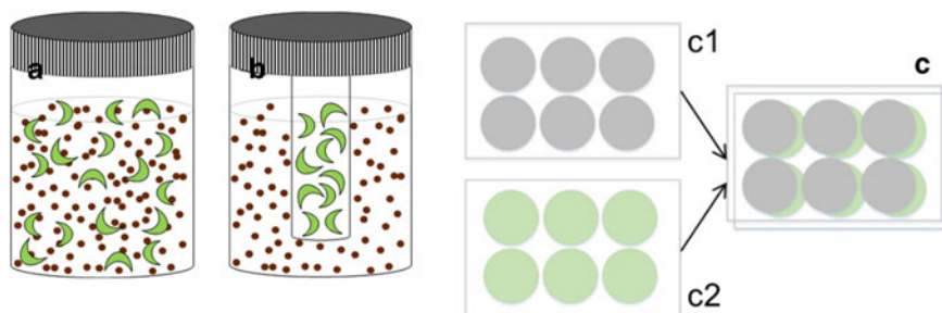
Fig. 15.2 Illustration of a testing setup for algal toxicity tests (a) and two setups to distinguish between physical and chemical effects of nanomaterials (b and c). In b, shading effects may be investigated using a double-vial setup, where algal cells are contained in the smaller inner-vial, surrounded by the nanoparticle suspension in the larger outer-vial. In c, the so-called “sandwich” setup reveals whether physical shading occurs in the algal test. Here one 6-well plate is filled with algal suspension without nanomaterials (c1) and another plate (c2) is filled with nanomaterial suspension without algae added. Plate c2 is placed on top of c1 and the combined “sandwich” setup is illuminated from above. For both modified setups (b and c), a decline in growth rate will be caused by physical shading caused by the tested nanomaterial (Modified from Sørensen et al. 2015). In addition to measuring growth rate (or biomass) in algal tests, changes in the algal pigment composition have also been a direct measure to quantify the effects of nanomaterial shading (Hjorth et al. 2016). This approach relies on the ability of algae to rapidly adapt their pigment composition in response to changing light conditions and therefore serves as an effective endpoint to quantify shading effects of nanomaterials (Hjorth et al. 2016)
